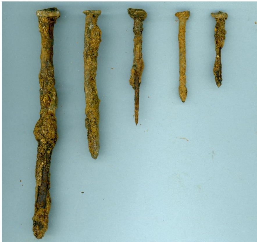
Figure 117. Top: Machine cut nails were most common in the fire deposits of House A, and included great variation in sizes. Bottom: Wire-drawn nails also were present in the fire assemblage, albeit in lower number and variety of sizes. The presence of the wire-drawn nails attests to remodeling activities on this dwelling during the very late nineteenth and early years of the twentieth century prior to the 1908 riots. All are actual size.
