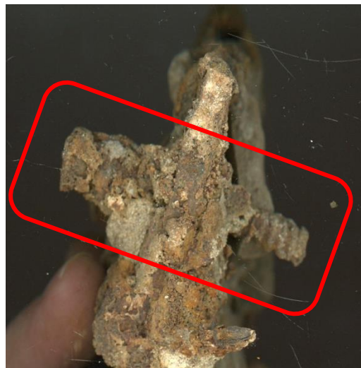
Figure 77. Top: Nails from the Fire Deposits of House B (Lot B-12) predominately were of the machine cut variety, and although the nails were generally fragmentary and heavily encrusted with plaster, three sizes were observed. These included heavy framing nails (4-in long), smaller framing and trim nails (2½-in long), and lath nails (1¼-in long) (Left). A small sample of clinched nails were also recovered, and probably indicates the presence of plank doors. Only one wire-drawn nail was recovered (right). Bottom: View of flat-tipped screw in butt hinge.
