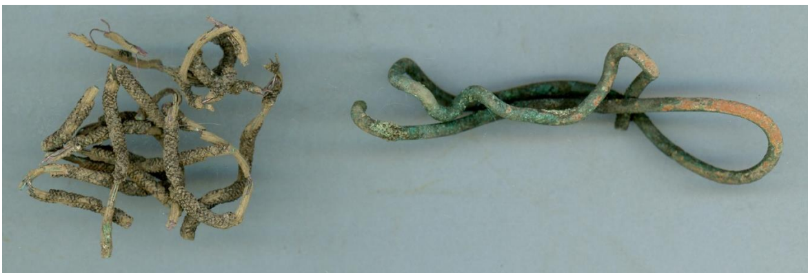
Figure 268. Electrical wire from House D. Left: Low voltage cloth-insulated wire (Lot D-84). Right: Heavy gauge, unsheathed copper wire (Lot D-21). Missing from this assemblage is any fragments of electrical porcelain.
