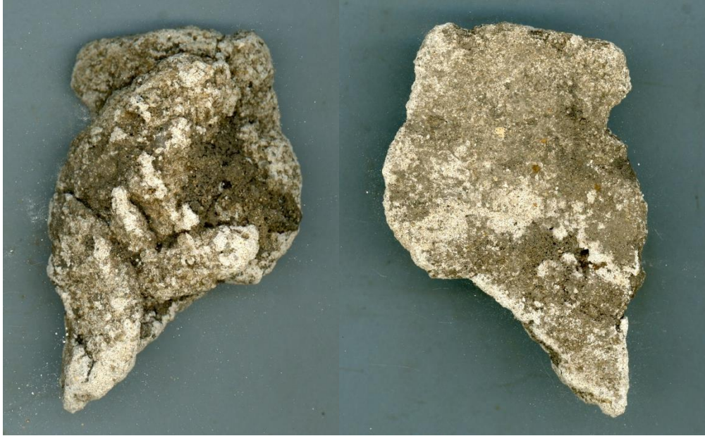
Figure 75. Plaster from the Early Pre-Fire component of House E. This plaster fragment consisted solely of brown coat (lacking any white coat). One surface was flat (but unfinished) whereas the opposite surface exhibited no evidence of lath “keys” and evidence of having been deposited as “droppings” (as if deposited wet in a wall cavity at the base of a wall after being extruded through the backside of a lathed wall, and initially representing construction waste). The presence of this artifact in the Early Pre-Fire deposits of House E suggests a relatively early remodeling episode that included the demolition and/or removal of actual walls (removal of walls and major remodeling activity) (Lot E-94; 75% actual size).
