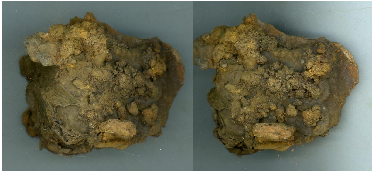
Figure 179. Two views of the trunk corner bracket or “clamp” (Lot E-144; actual size). Right: Note the tri-part lobed end of the bracket over-lying a sheet metal surface.
