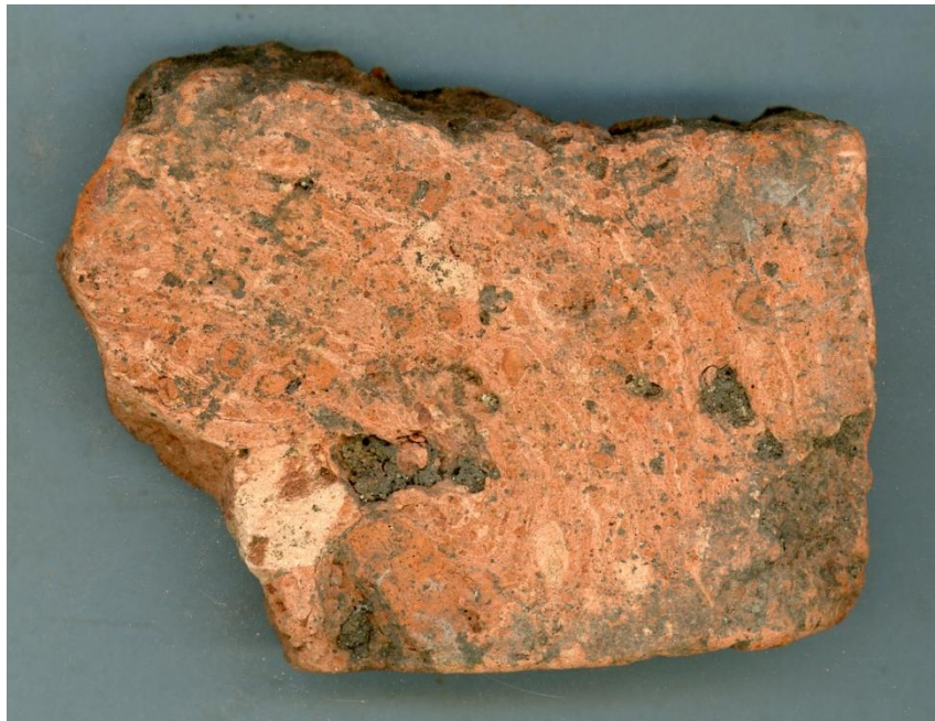
Figure 73. Paving brick, mottled paste; approximately 1" thick; molded into this form (Lot E-59) (actual size).
