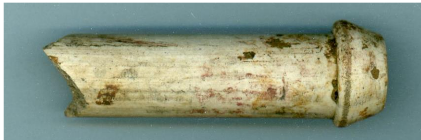
Figure 240. Architectural items recovered from Post-Fire context of House E include this porcelain “tube” for carrying electrical wiring through house framing (part of “knob-and-tube” wiring system) (Lot E-7)
