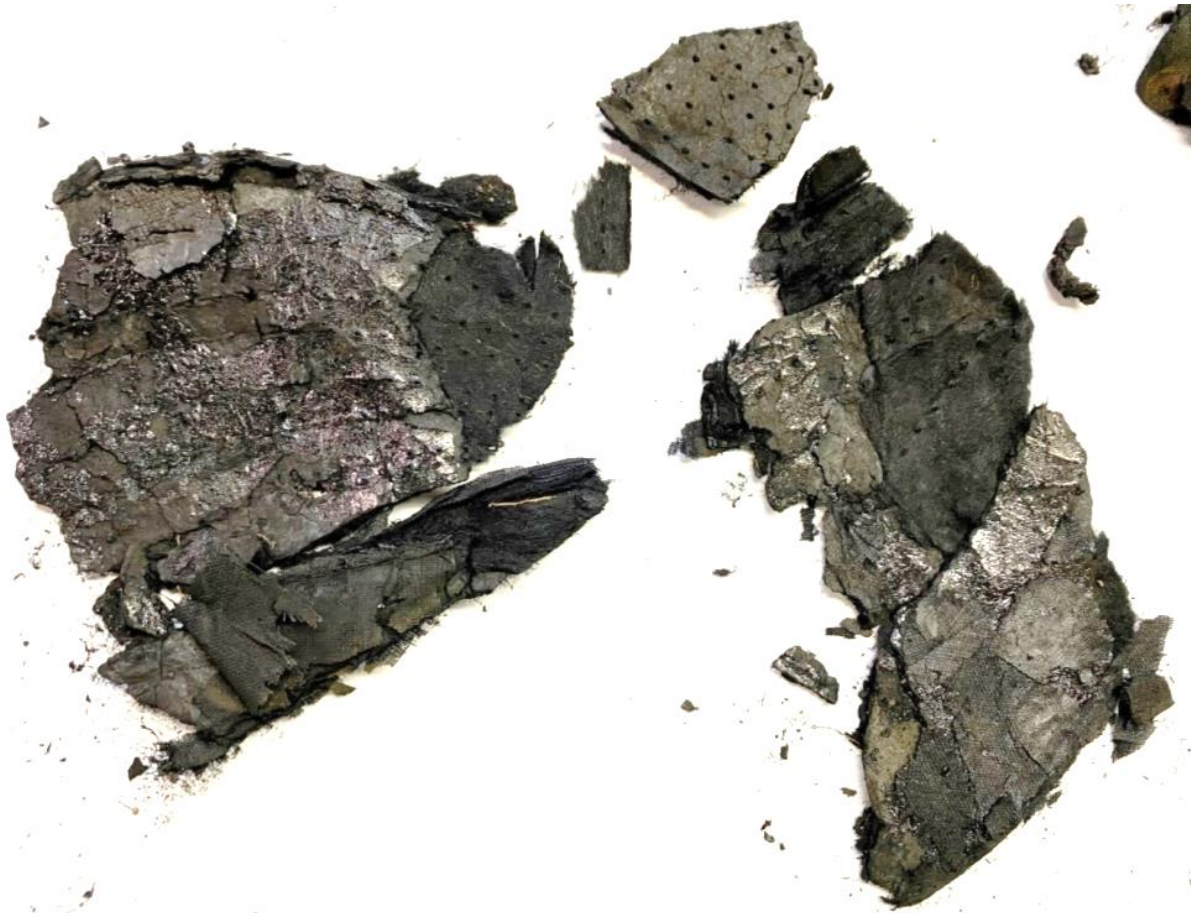
Figure 8: Textile 20. Nonwoven felt-like material. The shiny material may be heavily melted glue. The holes are remnants of heavy stitching.
