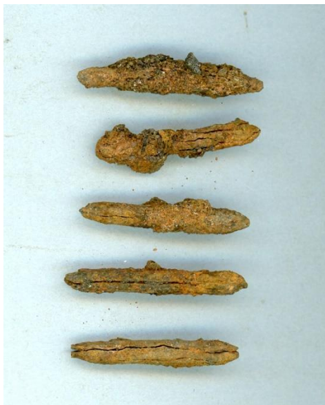
Figure 220. Potential fasteners consisting of double-pointed, wire-drawn “nails” and/or dowels which may represent fasteners used in furniture manufacture (edge joining of planks) (Lot E-98).
