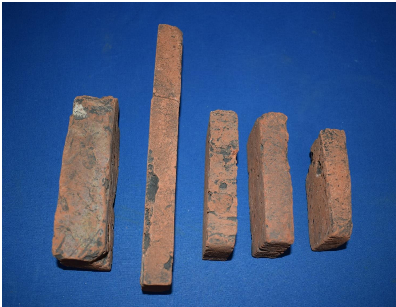
Figure 74. Fragments of sawn brick of unknown function. Most likely these brick were cut into this shape with the use of a hand saw. These brick were saw cut into “slabs” of variable thickness (ranging from \frac{3}{4} -in to 1\frac{7}{8} -in). The brick slabs were created by cutting along the long axis of the brick, as well as cut to various lengths along the short axis. These fragments were recovered from a front yard context (Lot E-191).
