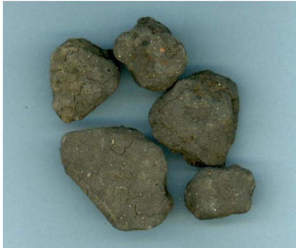
Figure 21. Small, dark-colored, low-fired, clay (?) nodules with sand inclusions potentially represent debris from an undocumented industrial activity (such as brick manufacturing) (Lot F-16). These fragments may represent highly weathered, extremely underfired brick. In this same context were recovered a coal clinker, and a large piece of fused window glass panes (Actual size).
